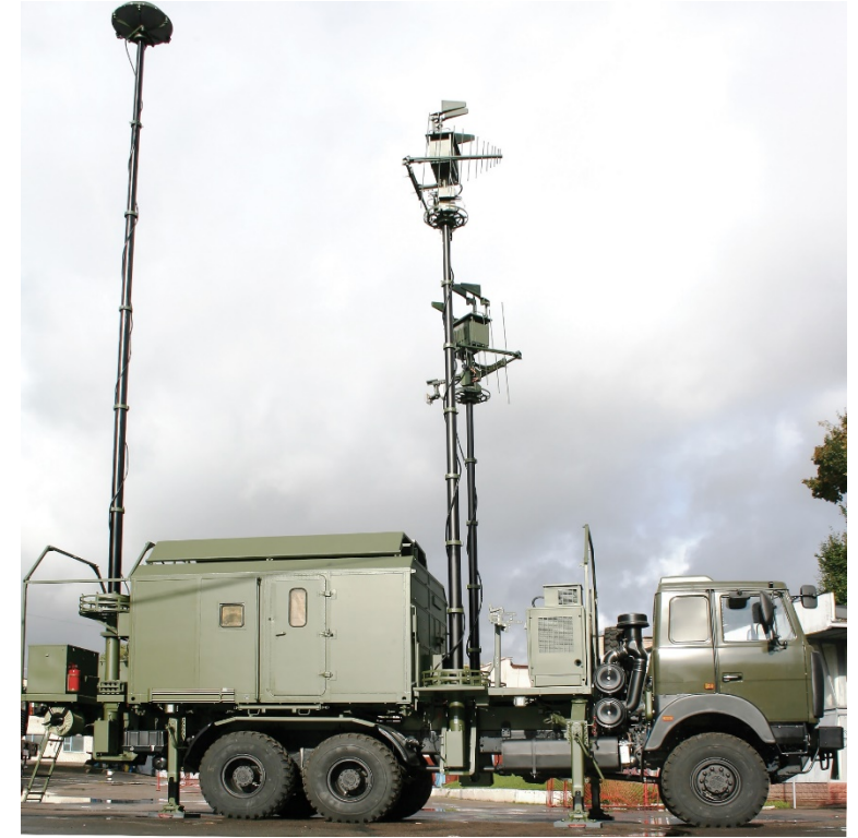
Mobile version for the Ministry of Defense and Border Guard – set of equipment installed on military truck with container for placement of the equipment and the crew
