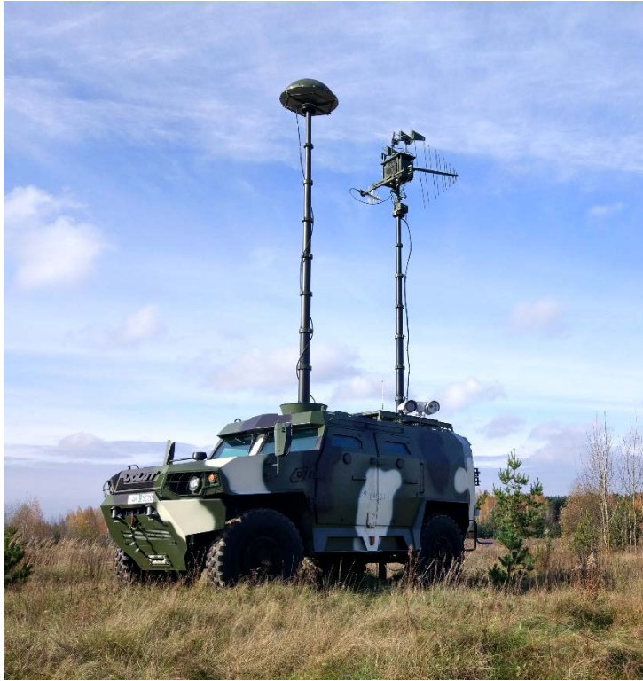
Mobile version for the Ministry of Defense and Border Guard – set of equipment installed on armored vehicle
